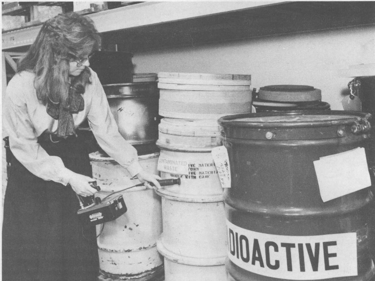
GLORIA CHAVEZ MILLARD (3202) uses radiation detector to check the integrity of stored drums of low-level nuclear waste awaiting disposal.
