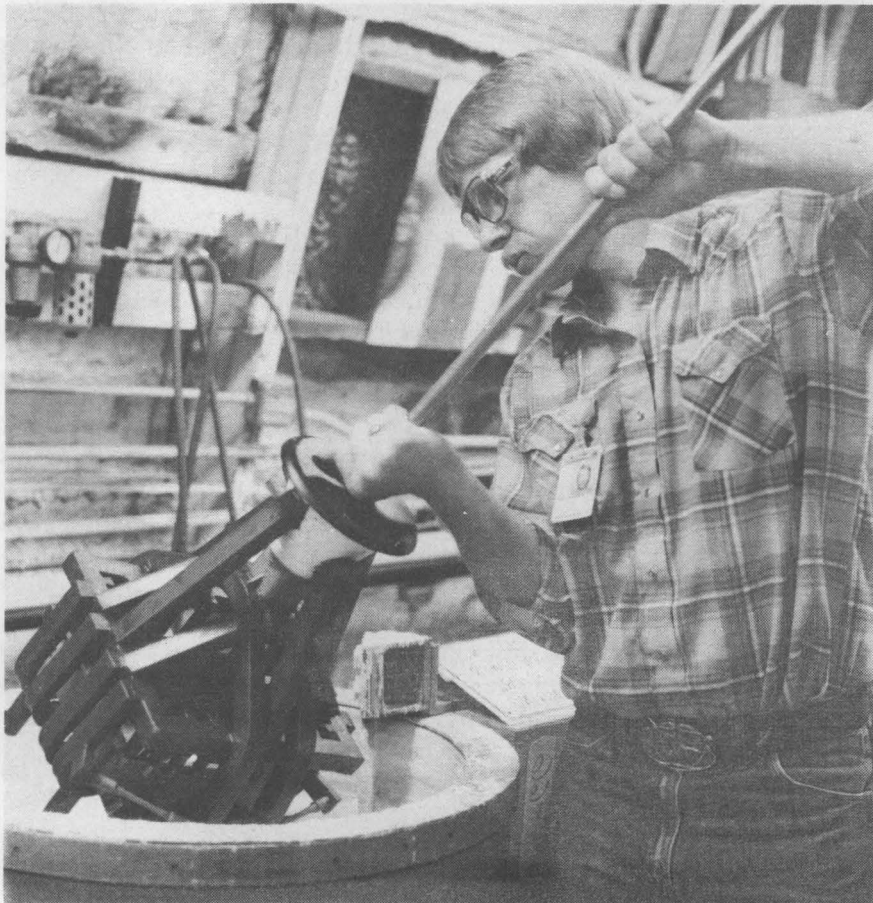
WAX PATTERN for B90 pre-flight-controller housing is dipped into ceramic slurry by Dave Toupal (7476). (Photo by Jim Bechdel, 3154)
