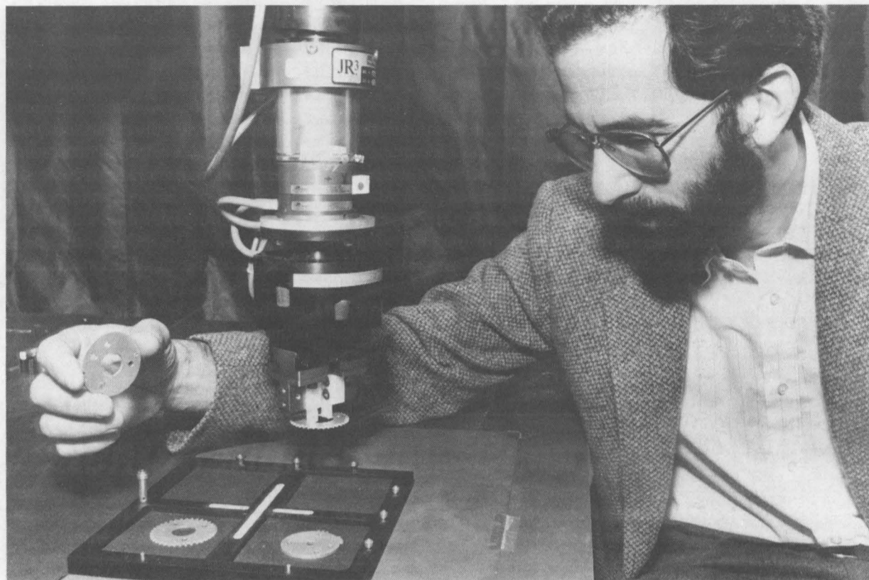
DAVID STRIP (1412) places parts in a "parts kit" that a robot (arm shown) picks up and assembles into a strong-link component. The robot uses an assembly plan that's developed by the Archimedes computer program. David and other Sandians in 1410 developed the program that allows a robot to program itself automatically to do mechanical assembly — believed to be the first program that makes this possible.
