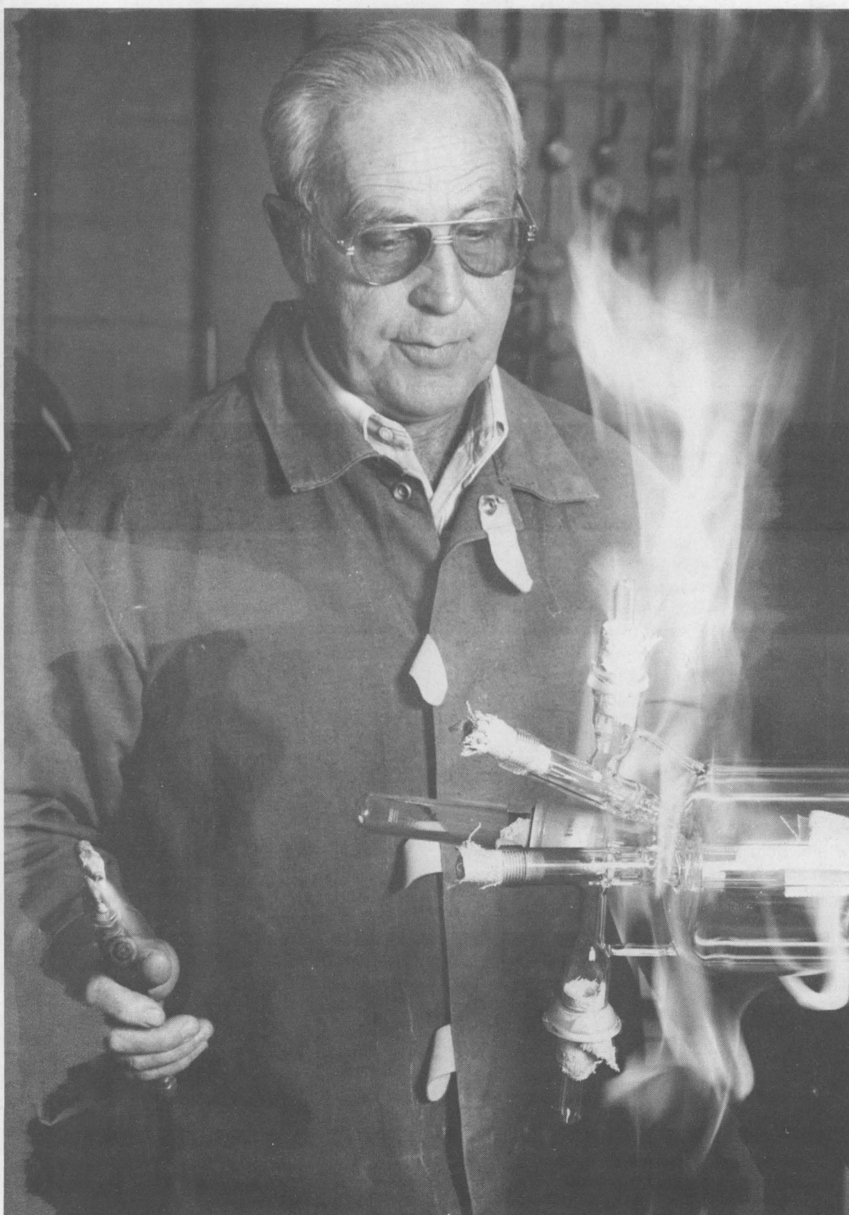
CLINT TUTHILL makes one of 24 recovery traps — each required to align perfectly with the others — destined for use in removing hydrocarbons from a vapor stream.
