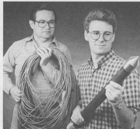
ART SENA, left, and Sandy Ballard (both 6231) display underground probe and cable designed to measure groundwater flow.
