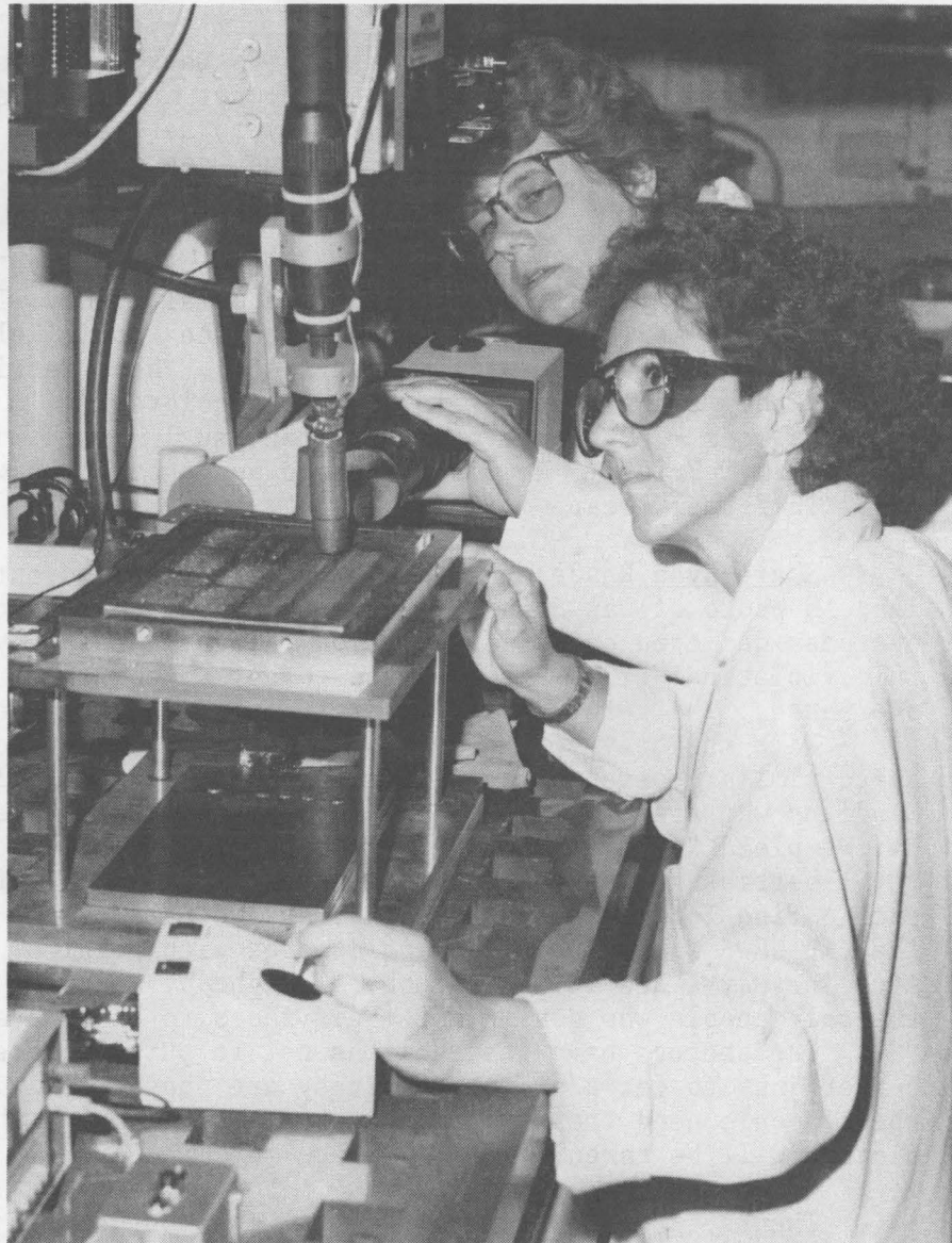
KIM MAHIN (8312, right) and Beth Fuchs (8342) prepare equipment for a welding experiment at Sandia, Livermore. The two are involved in the use of sensors to measure temperatures and displacements in real time during gas-tungsten-arc and gas-metal-arc welding.
