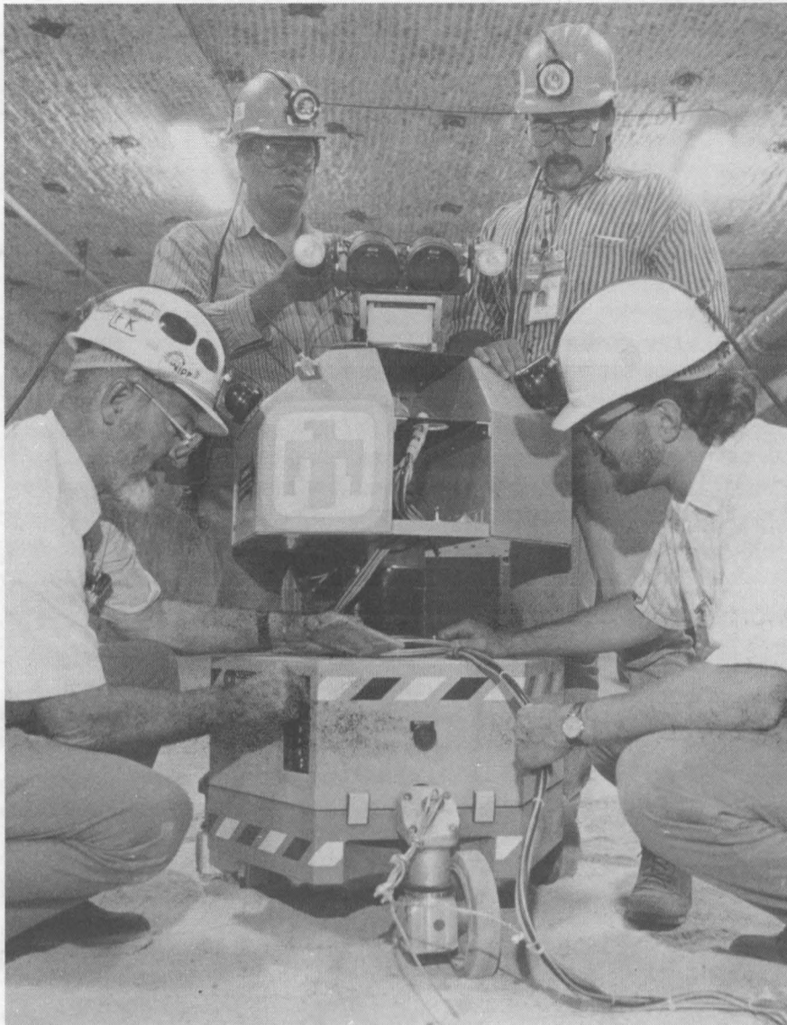
GIVING ROBO OP a final inspection before sending the mechanical Sandian into an underground test room are (from left to right) Tom Schultheis (6343), John Ortiz (9325), Mark Lemon (9325), and Tom Rice (2852). Robo Op's two video cameras provide researchers with an up-close view of the walls and ceilings of waste storage rooms that are too dangerous for humans to enter. The cable attached to Robo Op's bottom half carries electrical signals from the video cameras and helps researchers recover the robot if it tips over. (Photo by Jim Conklin, Westinghouse)
