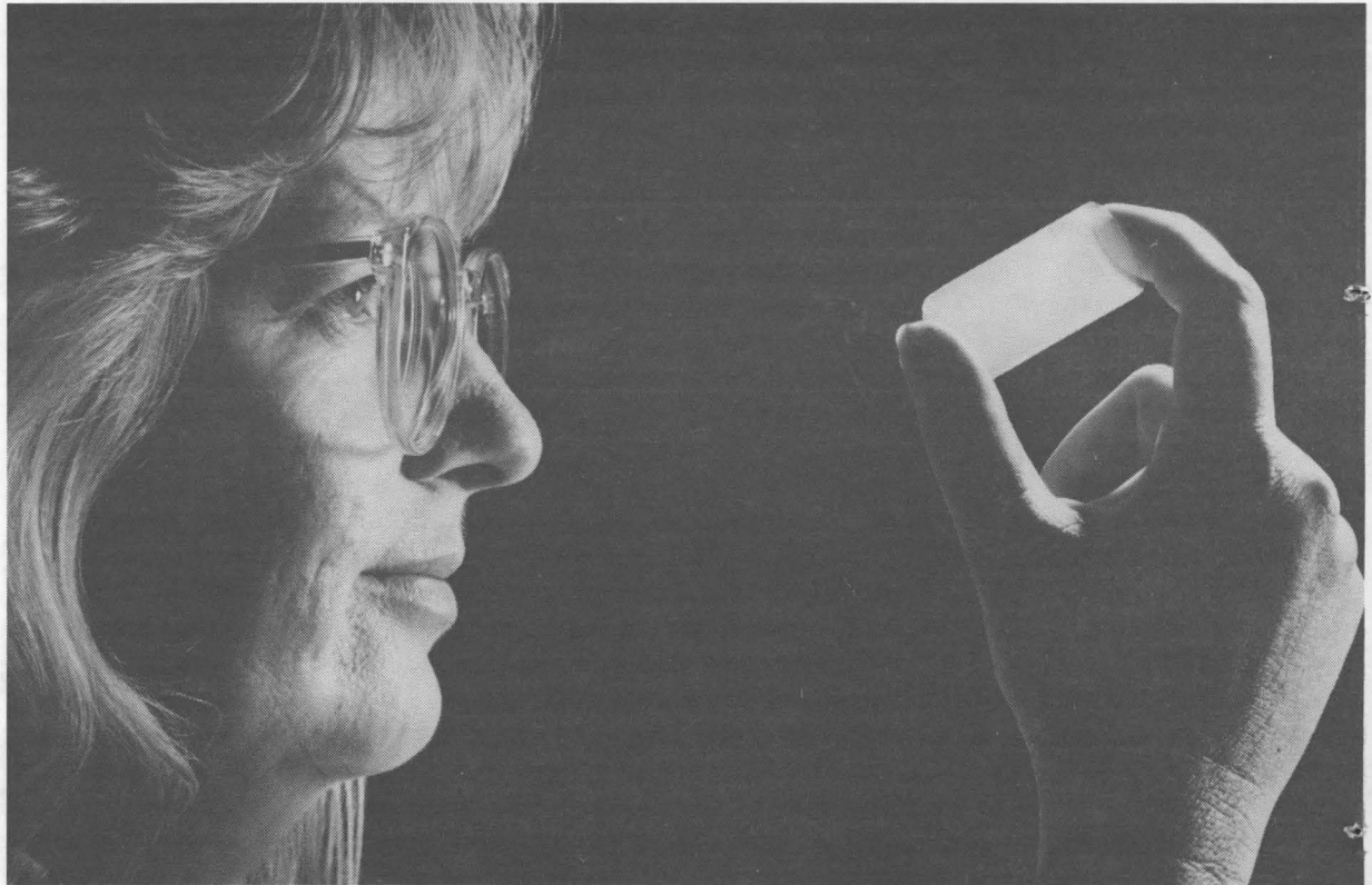
GLOWING GLASS — Carol Ashley (1846) gazes into a glass-like aerogel material used in new Sandia-developed radioluminescent (RL) lights. The solid-state Sandia lights glow up to 10 times brighter than conventional gas-filled RL lights. In the new lights, tritium and colored phosphors (simulated here) are chemically and physically trapped inside the plastic or aerogel solids. (Photo by Randy Montoya, 3162)
