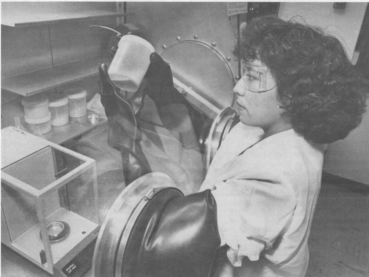
TERRI ZENDER (1842), a chemist, examines lead acetate to be mixed in solution, part of the procedure for producing ferroelectric thin films. The materials are kept inside an airtight chamber called the Inert Atmosphere Glovebox. The chamber is filled with argon gas and prevents materials from being exposed to air.
