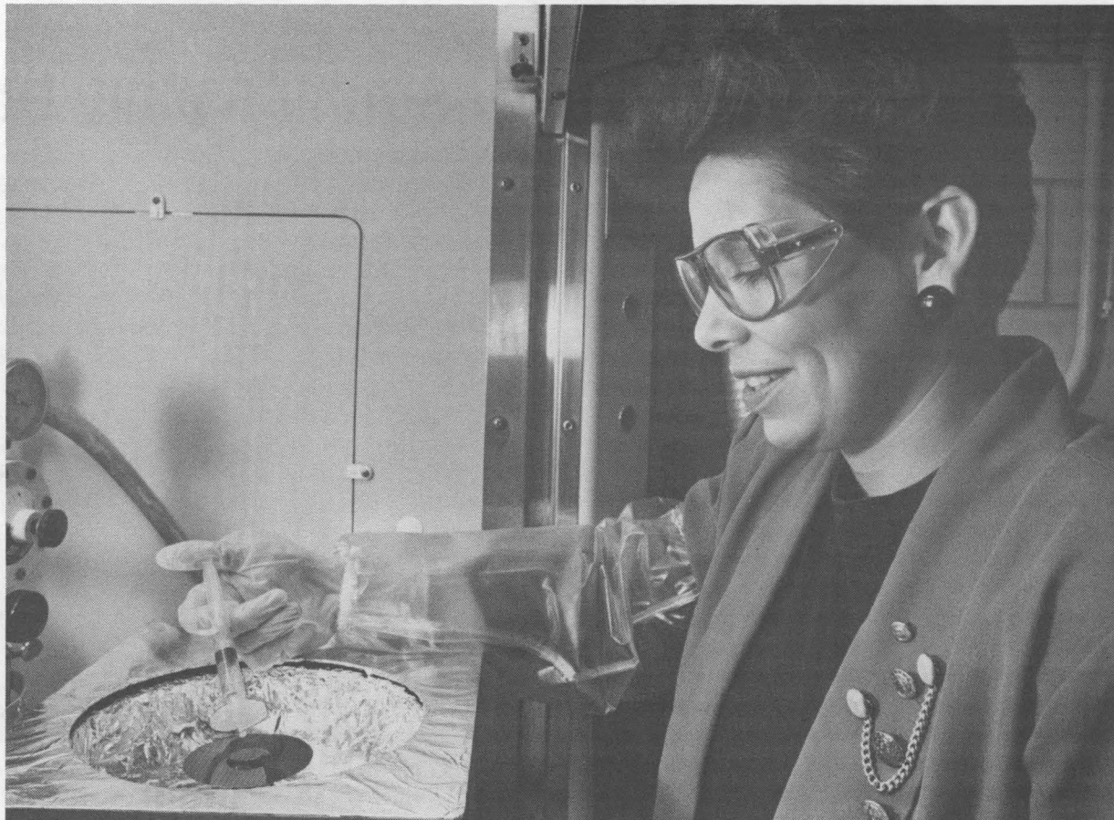
CINDY HERNANDEZ (1842), a chemist, squirts a small amount of solution onto a photoresist spinner, which turns at 3,000 rpm and distributes the film evenly across the surface of a photographically defined wafer.
