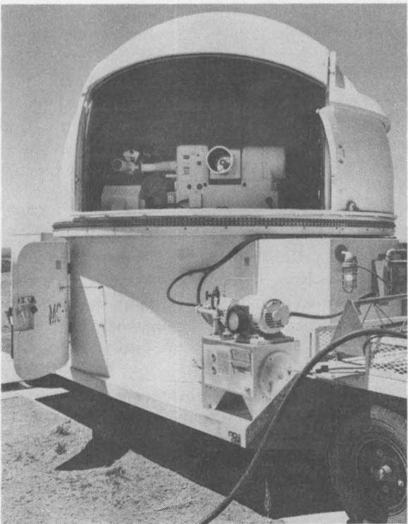
CINETHEODOLITE, with Ron Taylor (7514) at the controls, is at a precisely surveyed location and ready for tracking. The cinetheodolites can be moved from location to location for different test requirements and times of day.
