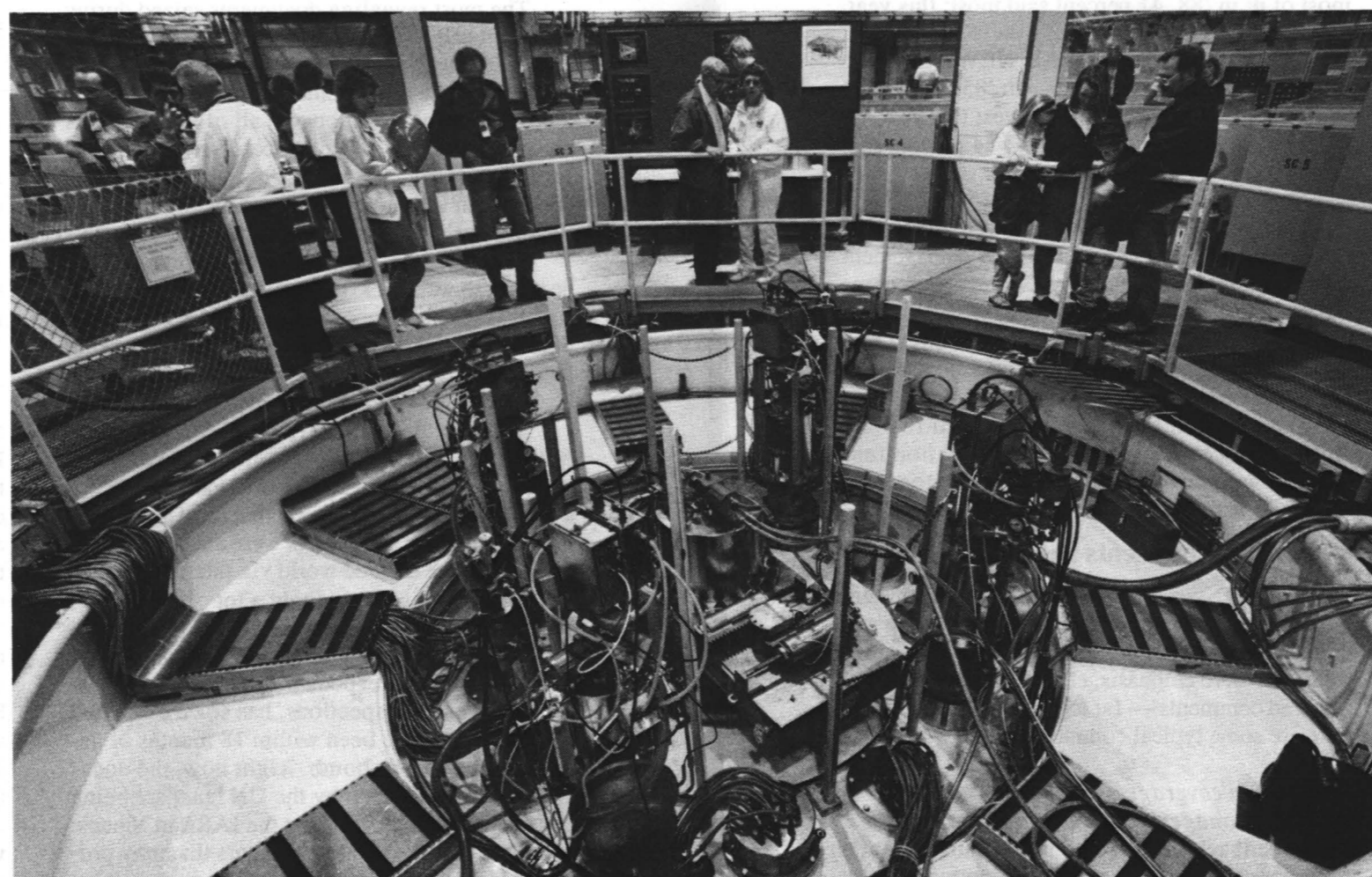
PBFA II (Particle Beam Fusion Accelerator) drew lots of Family Day spectators, who also got to watch divers inspect the facility after a test shot the night before. They were diving in the deionized water that insulates the components of the pulse-forming section of PBFA.
