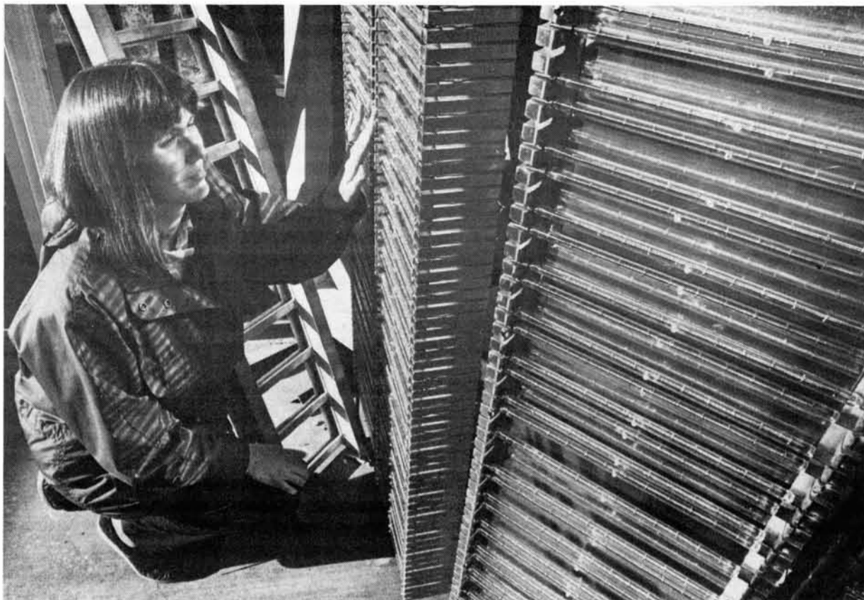
RADIANT HEAT ARRAYS , being examined by Keri Sobolik (2761), are the heat source for simulating hypothetical accidents in nuclear reactors. The array can simulate the heat that many different melt patterns would create. CYBL's double-boiler-like inner vessel can be subjected to heat as intense as 400 times the sunlight falling on a comparable surface. (Photo by Randy Montoya)
