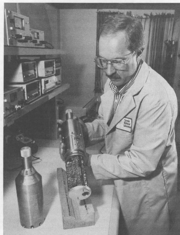
Jeff Morgan (2664) holds part of a downhole seismic sensor, developed at Sandia, like those that can be used to detect underground weapon tests.
