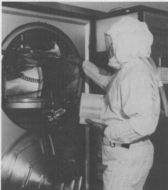
A WHITE-FROCKED lab worker extracts a 6-inch-diameter silicon disk from a metal deposition system in the Microelectronics Development Lab's Class 1 clean room.
