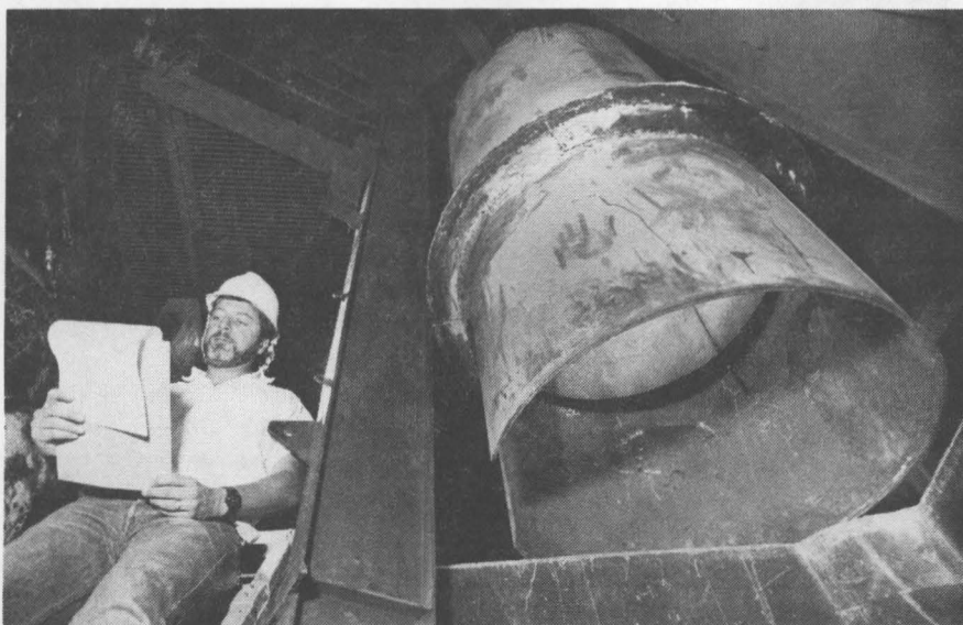
STEEL LINER for scale model of containment building looms over Marty Pilch of Severe Accident Phenomenology Dept. 6422. (Photo by Randy Montoya)
