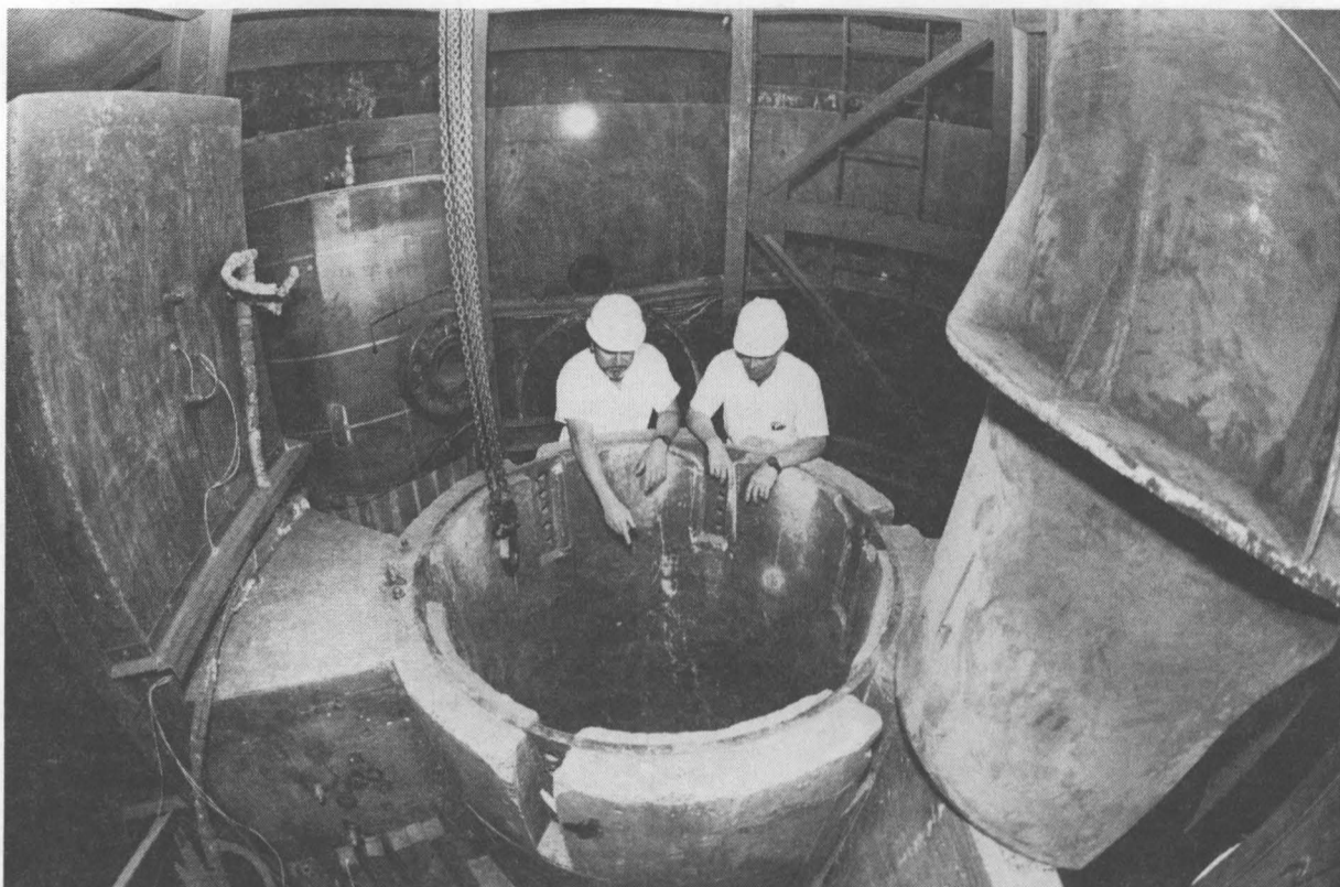
CONTAINMENT MODEL — Marty Pilch (left) and Michael Allen (both 6422) examine a containment structure at Sandia's Containment Technology Test Facility. A downsized version of the Surry nuclear power generator near Williamsburg, Va., the one-sixth scale model facility was used to test a severe type of accident that has never occurred in a power plant. (Photo by Randy Montoya)
