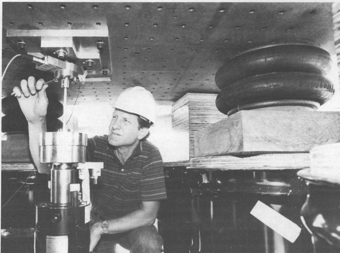
WHOLE LOTTA SHAKIN' GOIN' ON — When New Mexico State University researchers needed a bridge shaken up, they asked Sandia's Experimental Mechanics Dept. 2741 for help. On the old I-40 Rio Grande bridge, Randy Mayes (2741) tightens a connection between a hydraulic actuator and steel reaction mass used to do the shaking. The "tires" in the background are air bags holding up the 11-ton reaction mass. The bottom of the hydraulic actuator is bolted to the bridge, and the rod pushes repeatedly against the steel mass to produce the force for shaking the bridge. Test data relating the forces exerted by the Sandia shaker apparatus to deflection of the bridge has been compiled by Los Alamos National Lab for a New Mexico State study of damage detection in bridges. (Photo by Randy Montoya)
