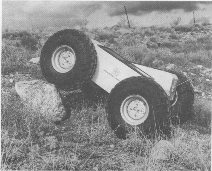
ONE OF THE two full scale (one-meter) working prototypes of the Robotic All Terrain Lunar Exploration Rover (RATLER) designed, assembled, and tested during FY93 goes through its paces on a Sandia test range. The RATLER system has logged approximately 15 hours of successful field operations in varied terrain (item on page 11).
