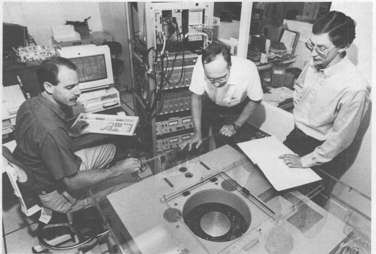
AN EXPERIMENT on a magnetically levitated positioner is done by (from left) Doug Jordan, Joel Darnold, and John Wronosky (all of Manufacturing Applications Dept. 2338). The technology could be used for ultra-precise applications, including integrated circuit manufacturing. (Photo by Mark Poulsen)
