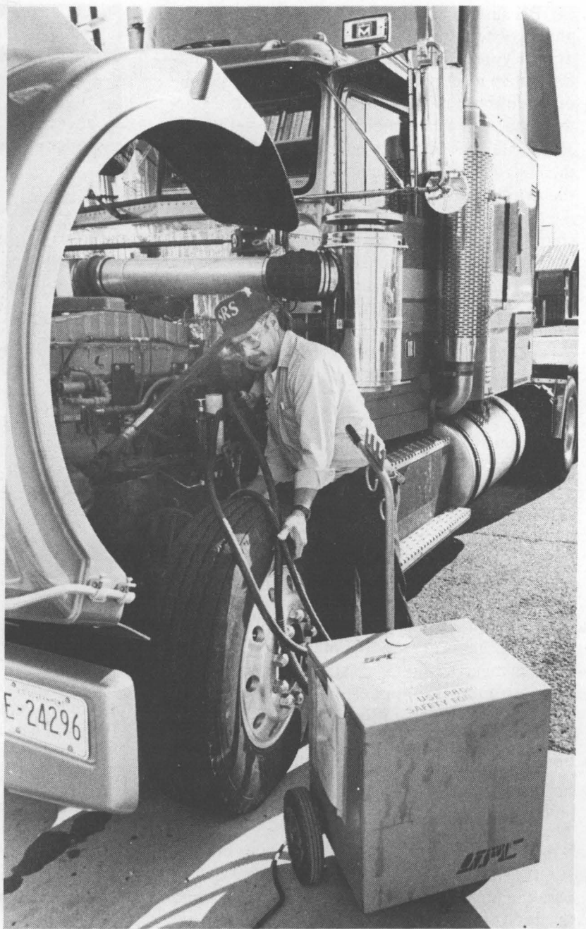
FRED RAETHER of Motor Pool Services Dept. 7614 connects a blender that takes oil from the crankcase of a DOE tractor, filters it, and mixes it with the tractor's diesel fuel. Recycling the motor oil saves money and avoids the environmental impact of disposing of it as a hazardous waste.
