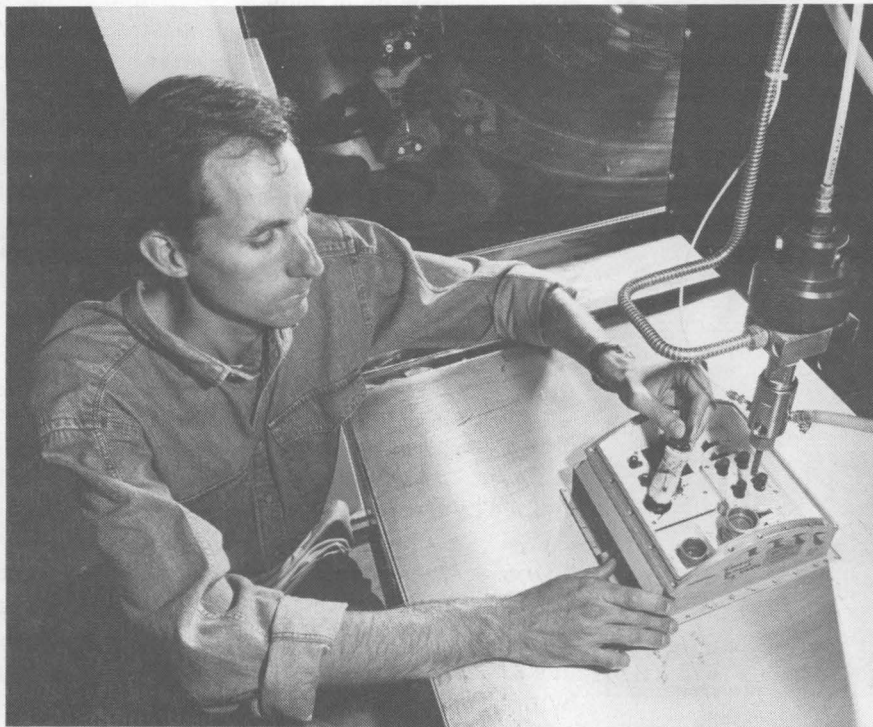
THE HAZARD-SEPARATION System cutting head (right) is shown in a lab test cutting a component from a piece of equipment, like the process that would be used to dismantle many nuclear weapon systems. Jim Lutz of Environmentally Conscious Life-Cycle Systems Dept. 6625 (left) examines the component after it is cut away from the larger housing unit. (Photos by Mark Poulsen)
