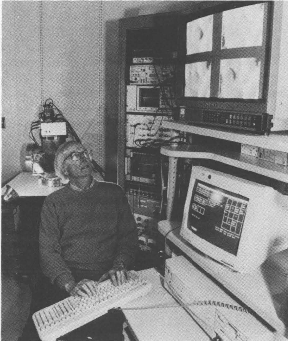
ATOMIC-SCALE IMAGING — Jack Houston operates keyboard controls of Interfacial Force Microscope he and Terry Michalske (both 1114) developed. The microscope vacuum chamber is at rear. The images on the system's video monitor illustrate the manipulation of individual nanometer-sized grains of gold in a polycrystalline gold film.
