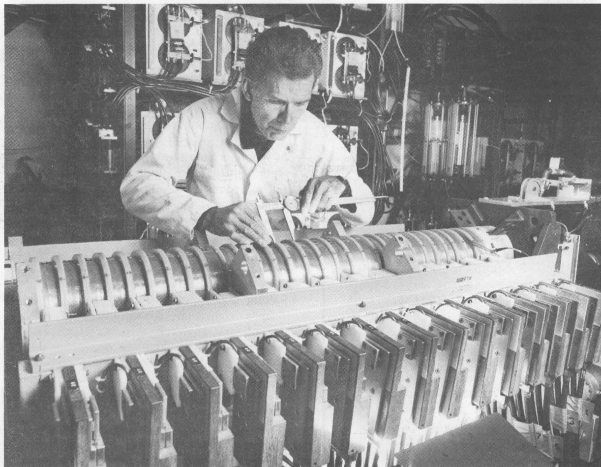
SANDIA COILGUN, a 35-stage version, is checked by Roque Feliciano, Jr. Electromagnetic Propulsion and Beams Applications Dept. 1221 is developing induction coilgun technology for a variety of potential military and commercial uses. (Photo by Randy Montoya)
