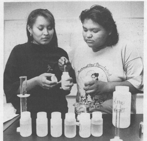
SAMPLING THE RIO GRANDE — Lisa Yazzie (left) of Tsaline, Arizona, and Janet Burbank of Chinle, Arizona, prepare Rio Grande river samples for testing as part of a College Bound water quality project. The samples will be exposed to varying amounts of chlorination for water purification purposes.
