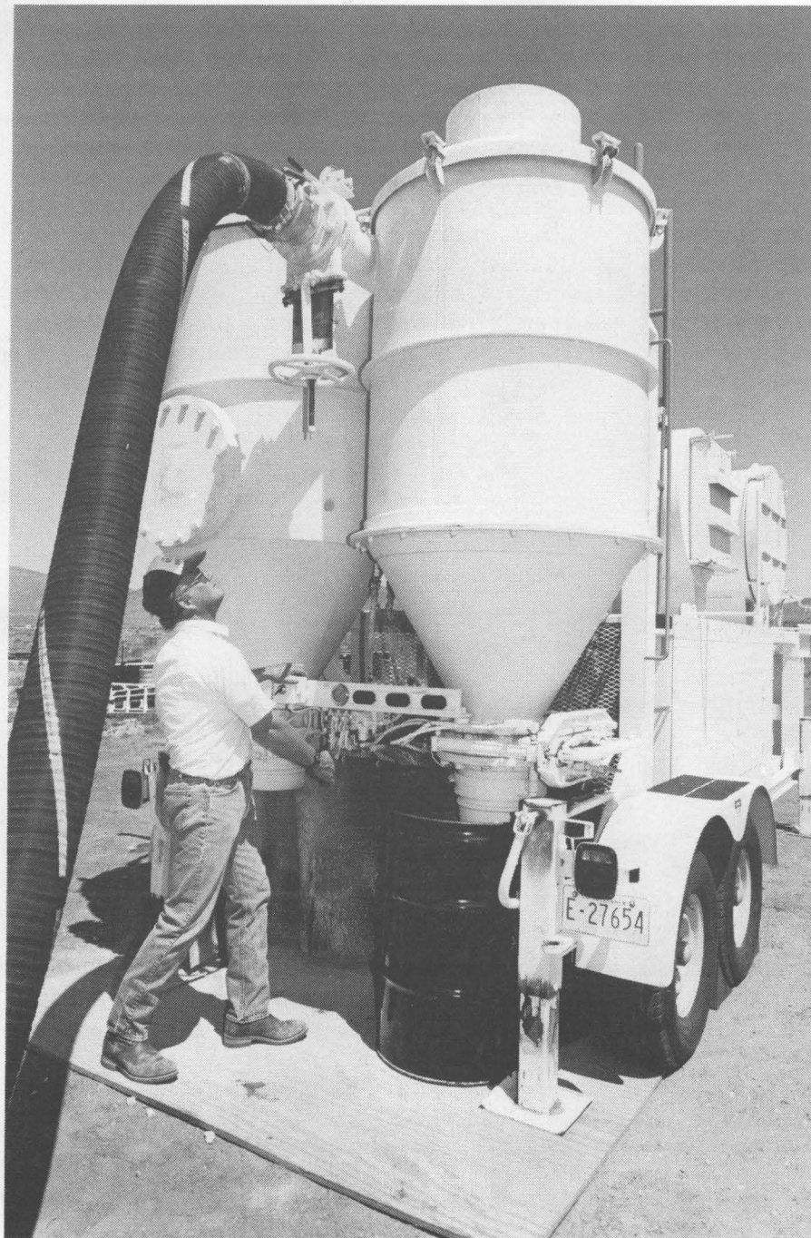
LARGE CLEANING JOB — Jim Westmoreland (6111A) adjusts controls on the vacuum and filter system that removes particles as small as 0.3 micron and volatile organic compounds from air drilling residue. Sandia and an asbestos abatement equipment company developed the system for use at environmental sites.
