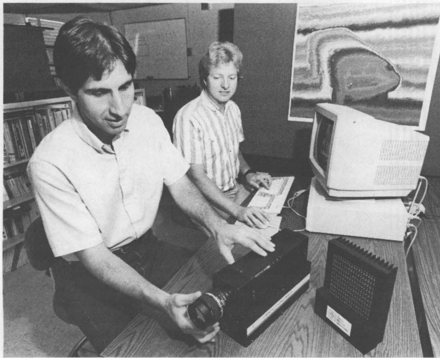
GETTING THE RANGE — John Sackos (left) adjusts lens on Sandia's scannerless range imager while Bart Bradley operates computer terminal. The system's light-emitting-diode array transmitter is at lower right. On the wall behind them is a range image of a missile-support vehicle. (Photo by Mark Poulsen)
