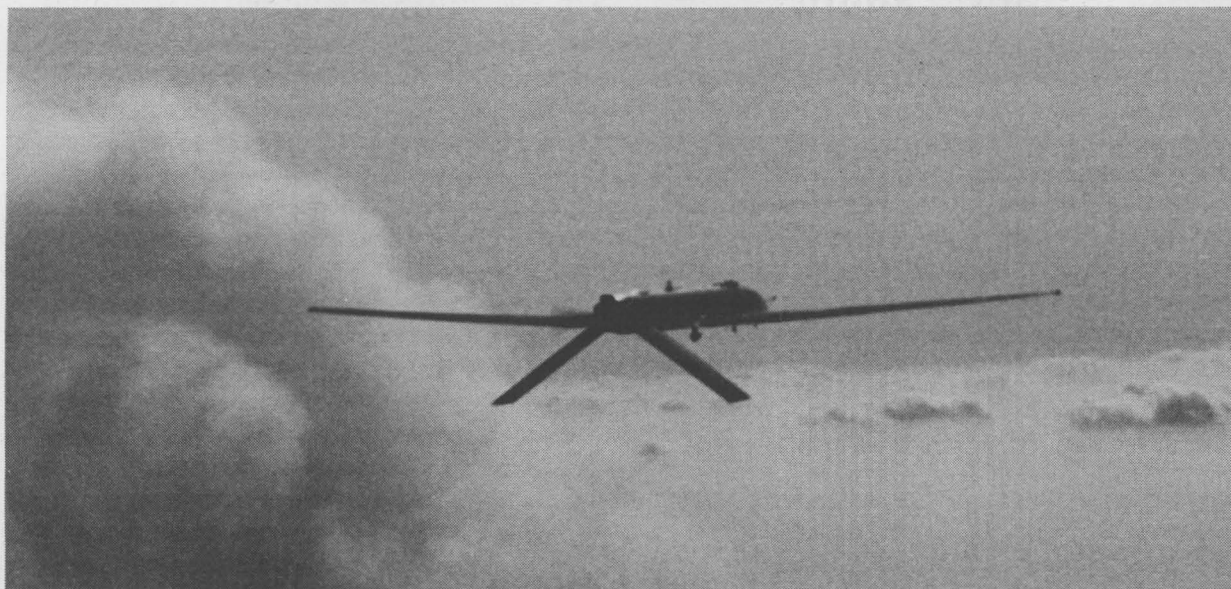
REMOTE SENSING — An instrumented, remotely piloted ARM-UAV (Atmospheric Radiation Measurement-Unmanned Aerospace Vehicle) collects data over Oklahoma in research aimed at improving understanding of the role of clouds in determining climate.
