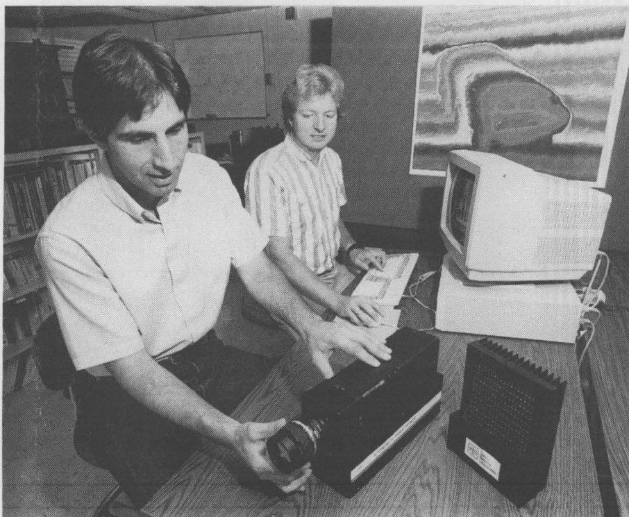
RANGE IMAGING — John Sackos (foreground) and Bart Bradley (both 9127) check components of a scannerless range imaging system developed by Sandia for Department of Defense non-nuclear weapon system applications. The system also has potential for many non-military applications.
