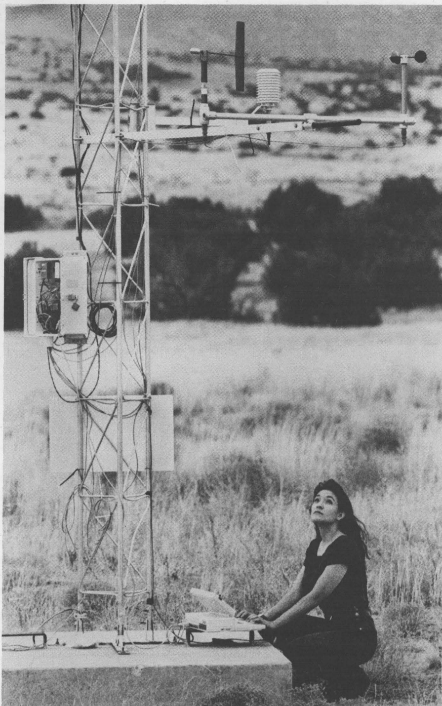
WEATHER WATCHER — Danielle Nieto (7575) downloads data from one of nine meteorological/ambient air monitoring stations that comprise Sandia's Clean Air Network. Among other things, the network will help establish background levels to show compliance with national ambient air quality standards.
