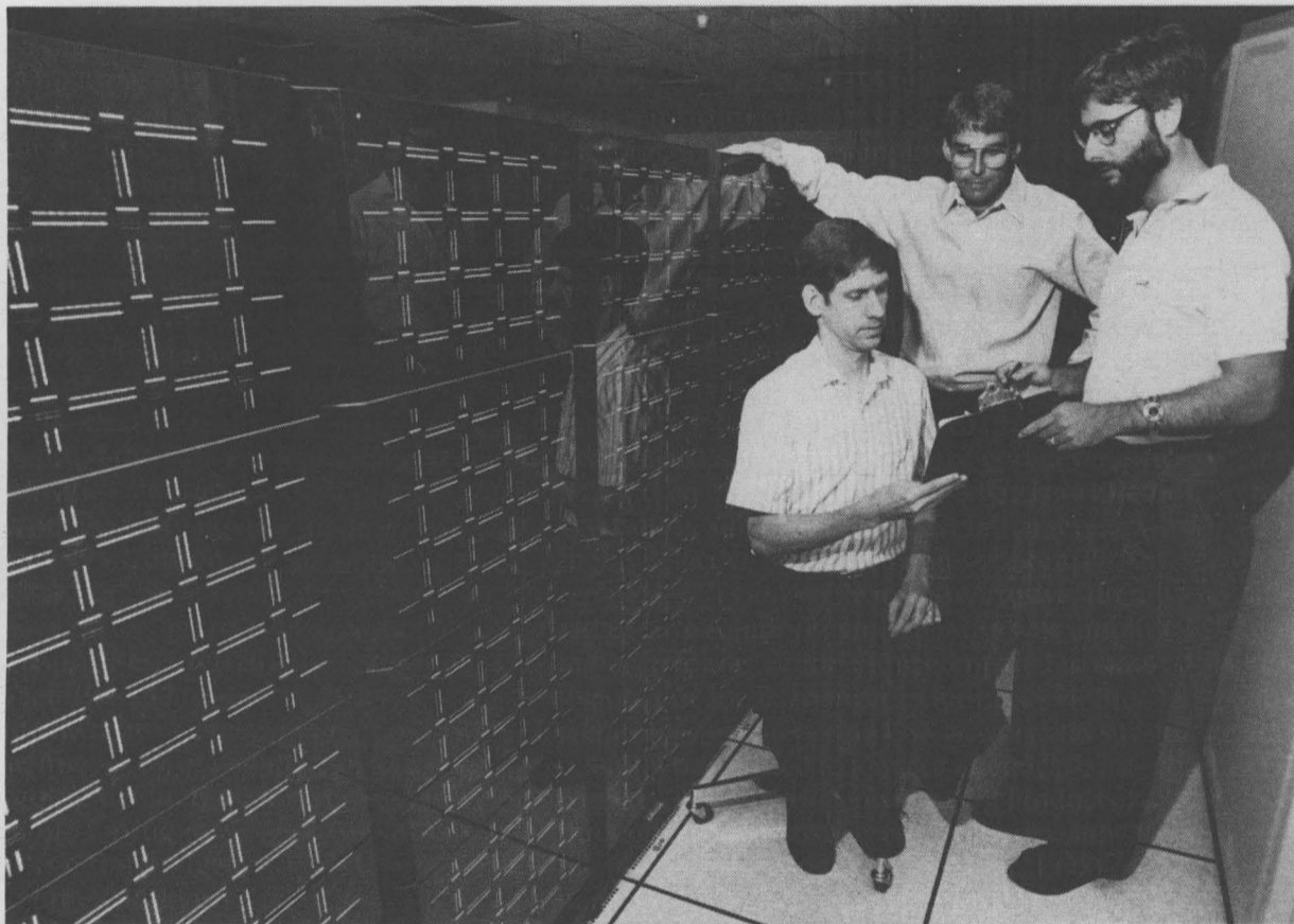
CHECKING RESULTS — David Womble (left, 1422), Art Hale (center, 1424), and David Greenberg (1423) check notes beside the massively parallel Sandia computer that set a record in May 1994 by performing 143.4 billion double precision floating point operations per second (Gflops/sec). The accomplishment won the Labs an R&D 100 award. They nearly doubled that speed in December 1994, with 281 Gflops/sec.
