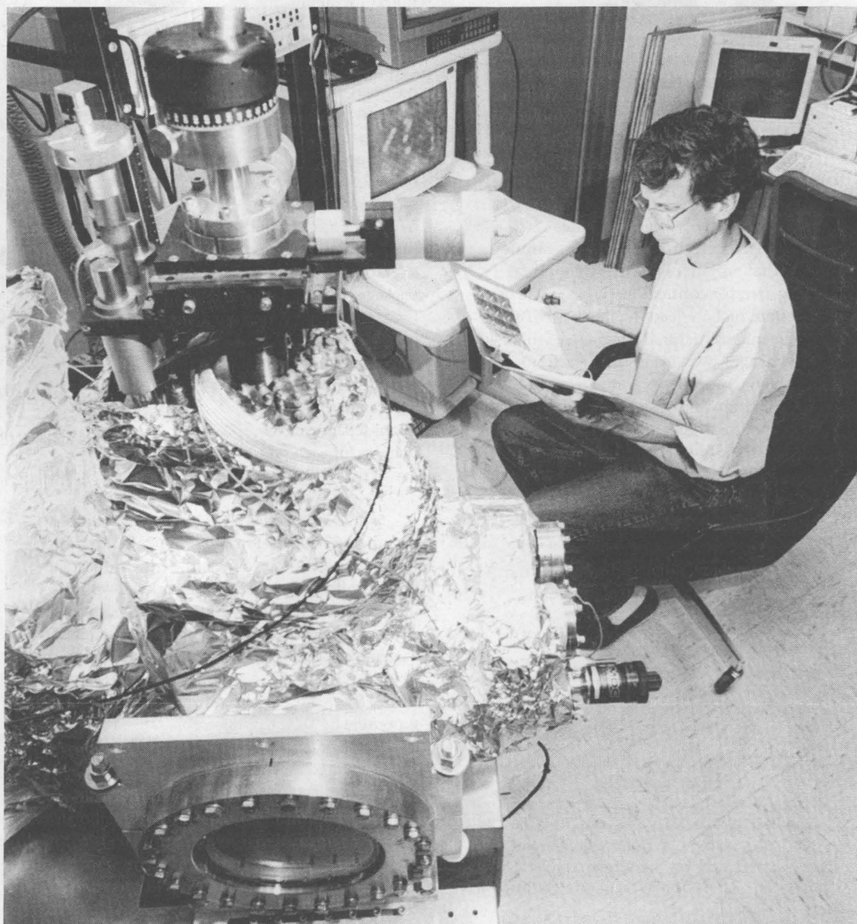
WATCHING THEM MOVE — Brian Swartzentruber (1114) at the scanning electron microscope he modified to track fast-moving atoms. His "atom tracker" is one of many accomplishments highlighted on this and the following pages. (Photo by Mark Poulsen)
