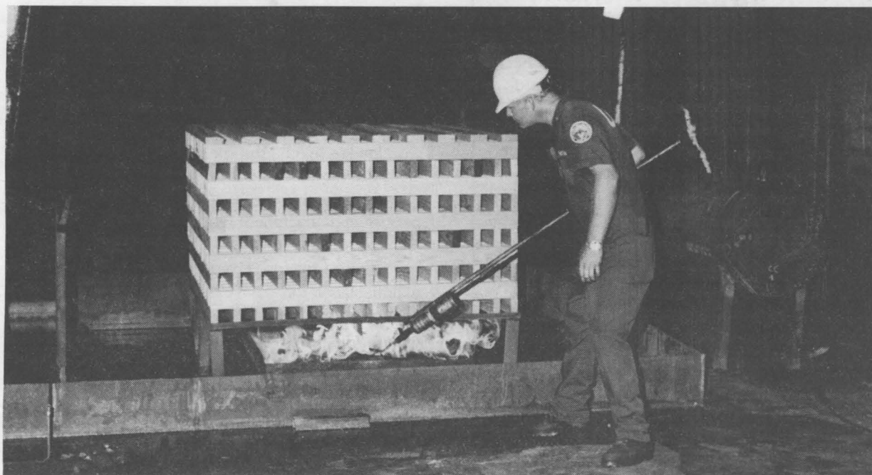
A BURNING ISSUE — Andrew Tinder, a member of the Coast Guard Fire and Safety Test Detachment at Mobile, Ala., ignites a wood crib aboard a Coast Guard ship in preparation for a SeaRAM test. (Photo by Diana Helgesen)
